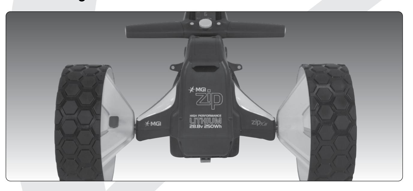
On the wheel, press the grey release button on the wheel hub. Place the wheel onto the axle. You will notice you need to match up the inner female groove on the axle and the male of the wheel. When placed in position simply release the button. You will notice you hear a "click" when the wheel is properly secured. To check that the wheel is properly in position pull on the wheel. If it is properly in position it will not slide off. Repeat for the other wheel.
