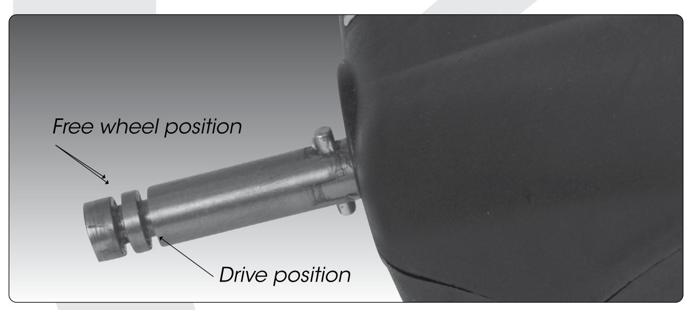
i. Drive position – Lock the wheel onto the groove closest to the battery base. To do this, press the grey release button on the wheel hub, push the wheel on to the axle as far as possible. To test for drive position try rolling the wheel backwards. If you feel resistance then the wheel is now in drive position and ready to use. Repeat for both wheels.
