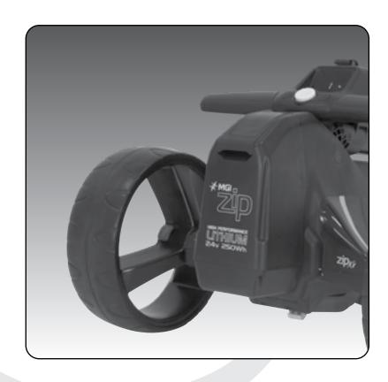
Push the handle down to connect the battery to the Zip X5.
